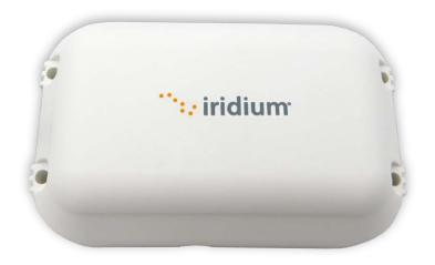
Iridium Edge is a satellite IoT communications device that can be rapidly deployed and complements terrestrial-based solutions to create worldwide connectivity.
